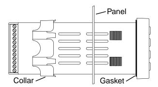
From the rear of the panel slide the mounting collar over the housing. Hold the housing with one hand and using the other hand, push the collar evenly against the panel until the spring loops are slightly compressed. The ratchets will hold the mounting collar and housing in place. To remove, gently lift the ratchets and slide a piece of heavy paper or mylar sheet under each ratchet (a business card works well). Slide the collar off of the housing.
